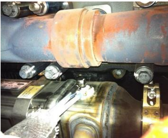
Figure 4. Rear Accelerometer Position on EGR Cooler
