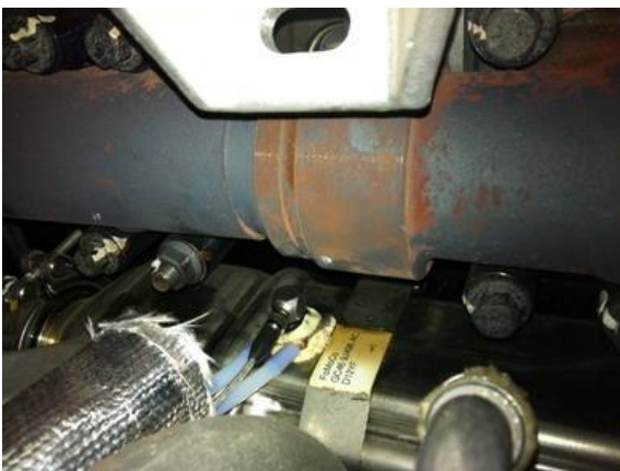
Figure 3. Front Accelerometer Position on EGR Cooler
