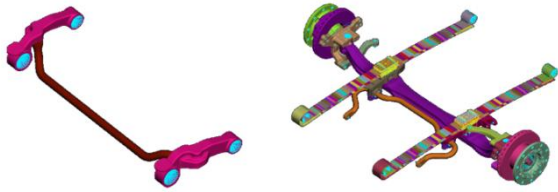
Figure 4. FE Model of Cabin Anti Roll Bar and Front Suspension Model
