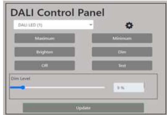
Fig.23. DALI Control Unit User Interface
