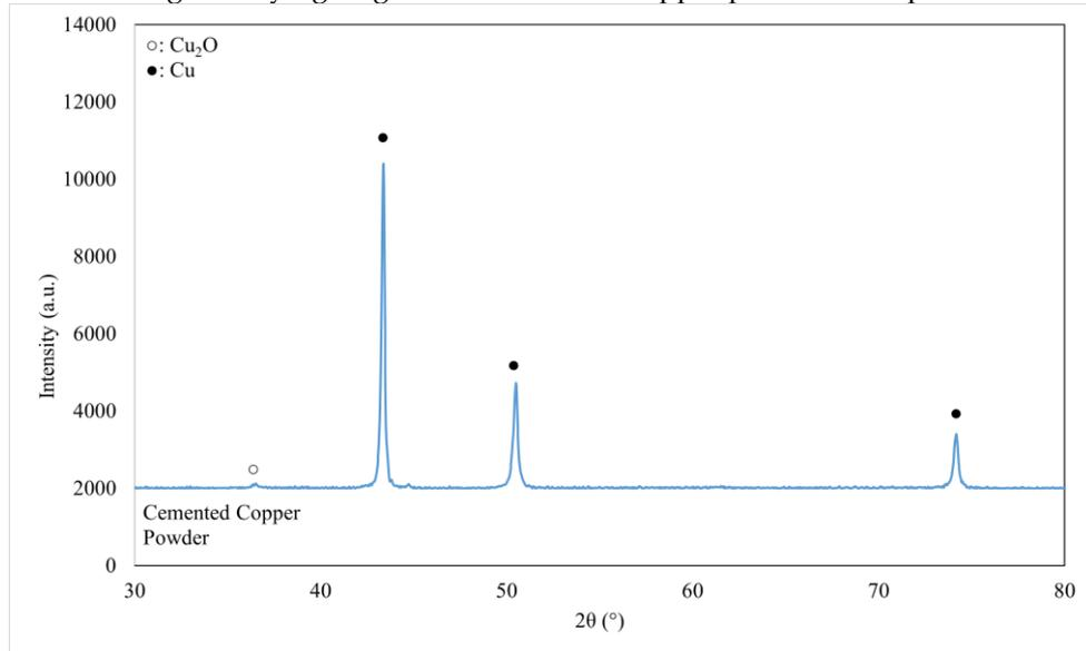
**Figure 6.** XRD graph of cemented copper powders.
