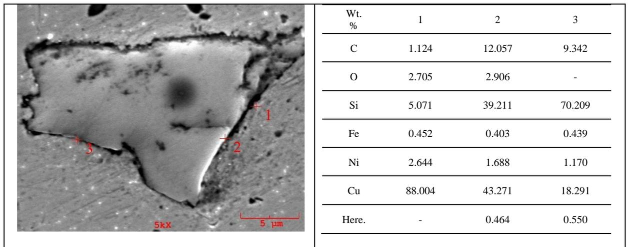
**Figure 10.** SEM-EDS analysis of cemented Cu-0.5wt.%Ni SiC composite
