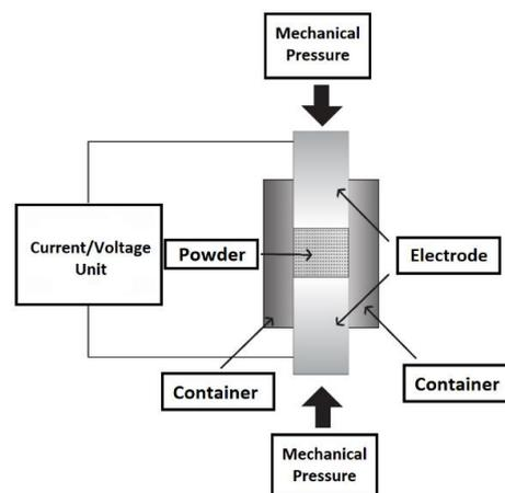
**Figure 3.** Schematic representation of sintering by ECAS Method [11], [15].
