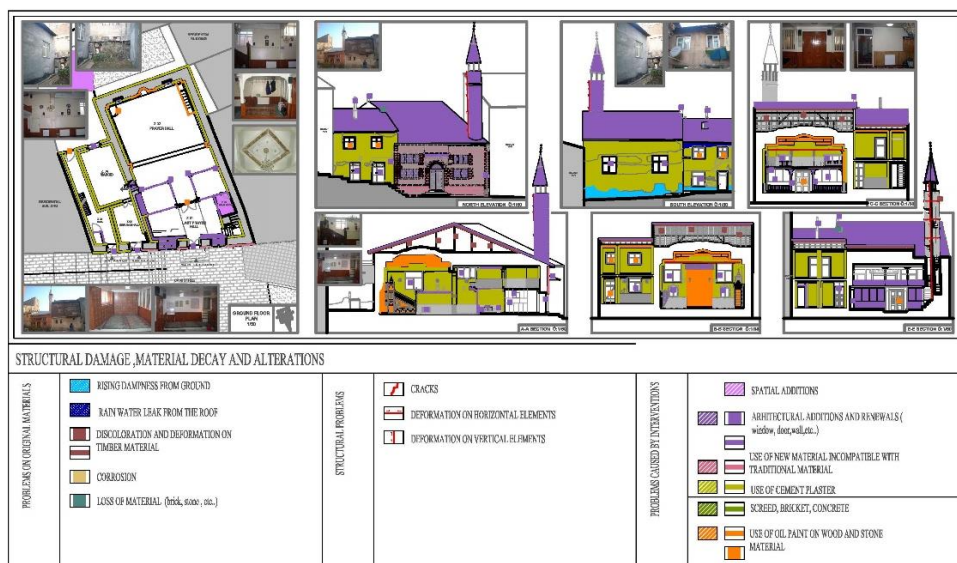
Figure 9. Problems detected in the whole building
