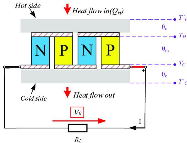
**Figure 1.** Structure of the thermoelectric generator
