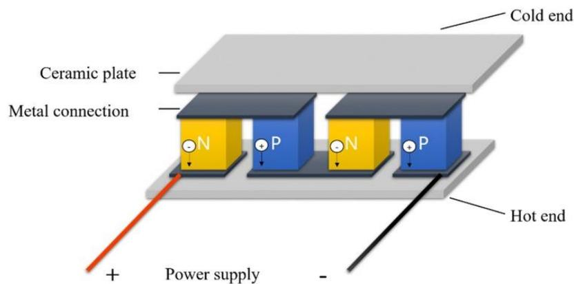
**Figure 3.** Internal structure of the thermoelectric module
