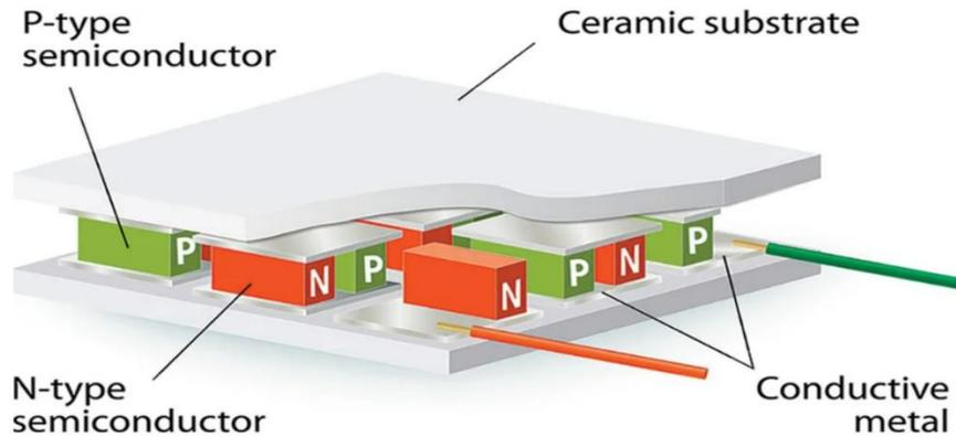
**Figure 2.** Internal Structure of Thermoelectric Module
