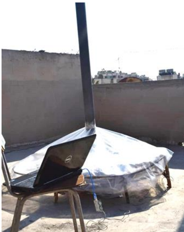
Figure 1. In-house- built a prototype of a SCPP.
