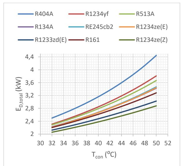
**Figure 17.** Variation of the  $E_{D,total}$  with the condenser temperatures of the refrigerants
