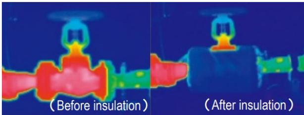
Figure 1. Effect of insulation
