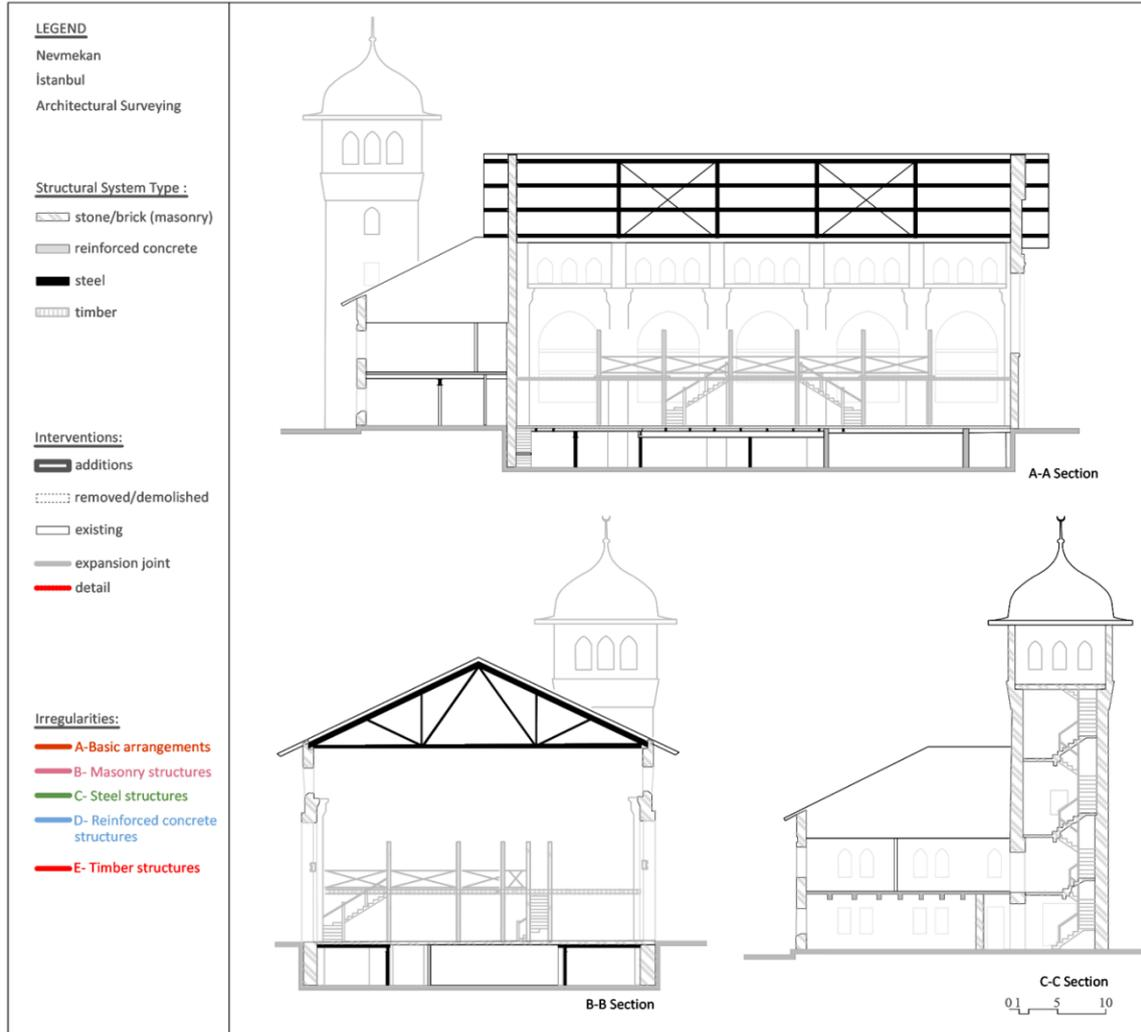
Figure 11. Nevmekean restoration project sections (Adapted from Köroğlu, 2019)
