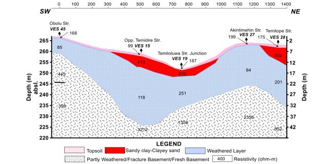
Fig. 4. Geologic Section/Profile along the selected VES point established in the study area
