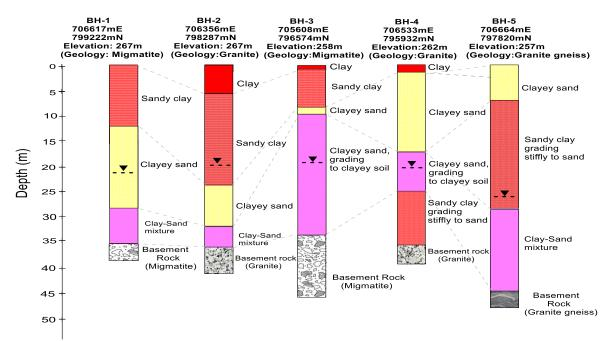
Fig. 7. The borehole sections across the study area, in granite, migmatite and granite gneiss environments
