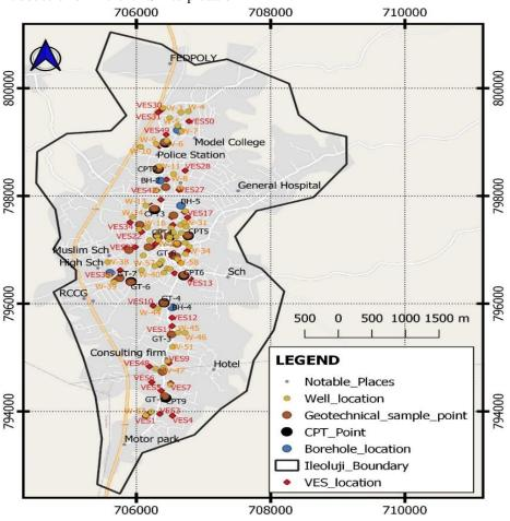
Fig. 3. Data Acquisition map for the study showing sample locations for geotechnical/geochemical and Field Survey
