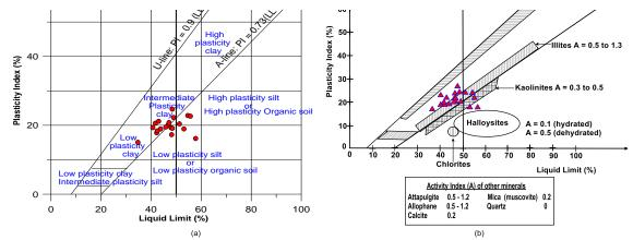
Fig. 8. (a) Plasticity Chart for the soil samples, showing prominent CL and CI plasticity group (b) Clay mineralogy group of the soil samples with most within Illite group
