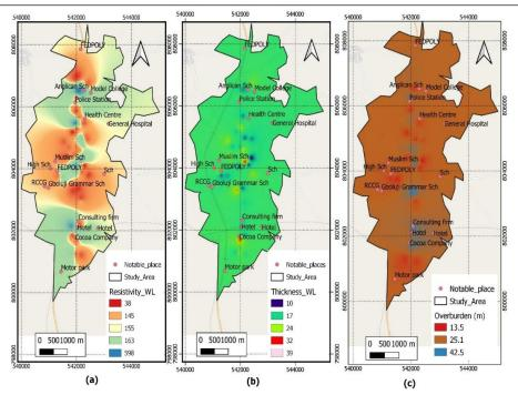
Fig. 5. Spatial Distribution Map of (a) weathered layer resistivity (b) weathered layer thickness (c) overburden thickness across the study area
