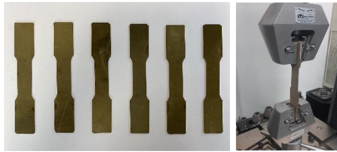
Figure 3. Tensile Test a) Samples b) Real Conditions Test
