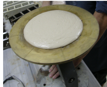
Figure 3: Flow table test result of AAP with Type II NaOH at lesser S/P ratio
