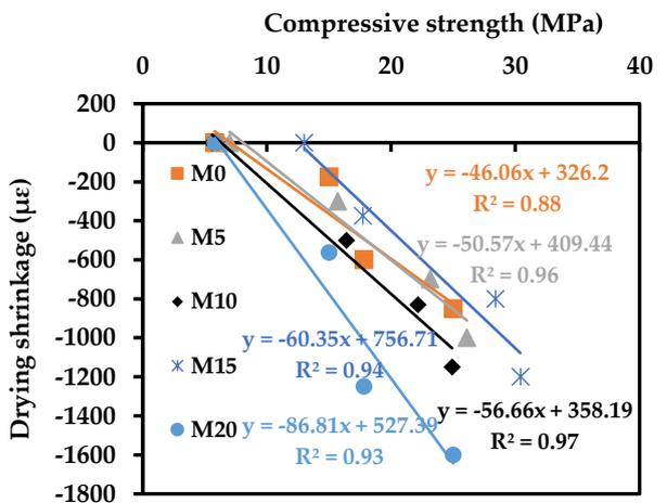
**Figure 12:** Correlation between compressive strength and drying shrinkage for mortars containing different percentages of LF.
