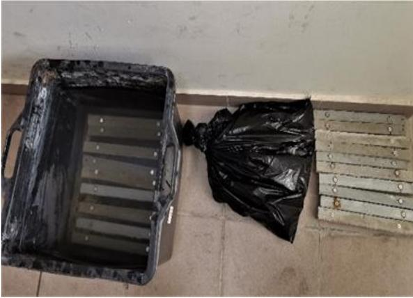
Figure 2: Drying shrinkage, autogenous shrinkage and expansion samples.
