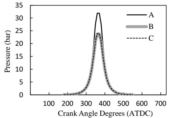
Fig: Calculated cylinder pressure versus crank angle compared for three pistons.
