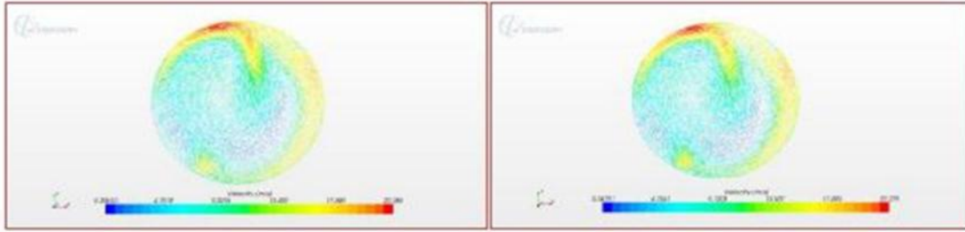
Fig.6 Steady and Unsteady Simulation Results on Midplane of the Engine Cylinder.
