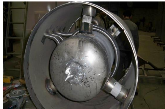
Figure 2.2. Nested Inner and external tanks
