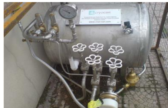
Figure 2.3. LNG Autogas filled with LNG and mounted to experiment set
