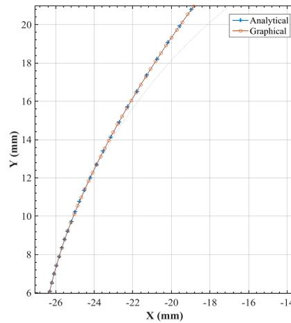
**Figure 8.** Left middle region view of two profile data produced by analytical and graphical approaches - flat face follower cam profile
