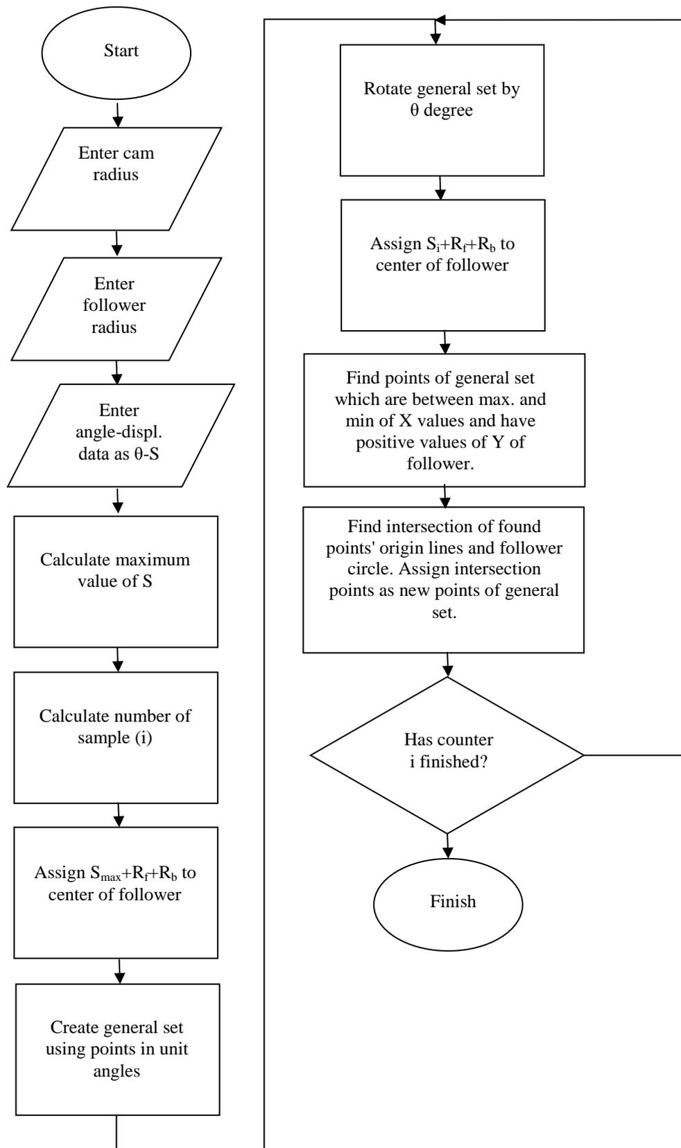
**Figure 4.** Graphical approach algorithm for roller follower cam mechanism
