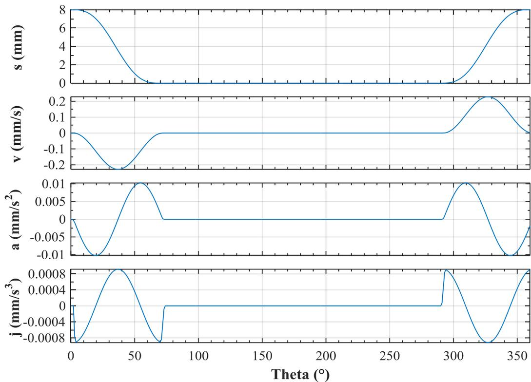
**Figure 5.** Kinematic graphs of used displacement data
