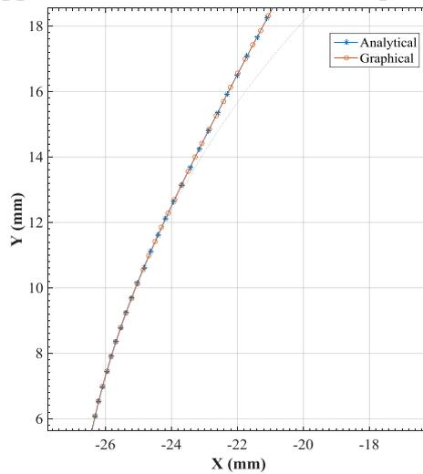
**Figure 12.** Left middle region view of two profile data produced by analytical and graphical approaches - roller follower cam profile
