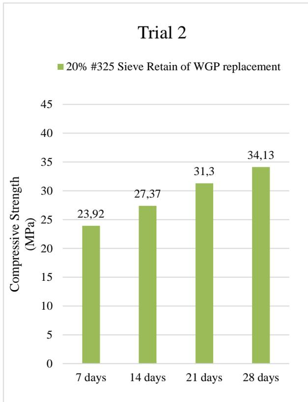
Figure 6: Trial 2 Compressive Strength
