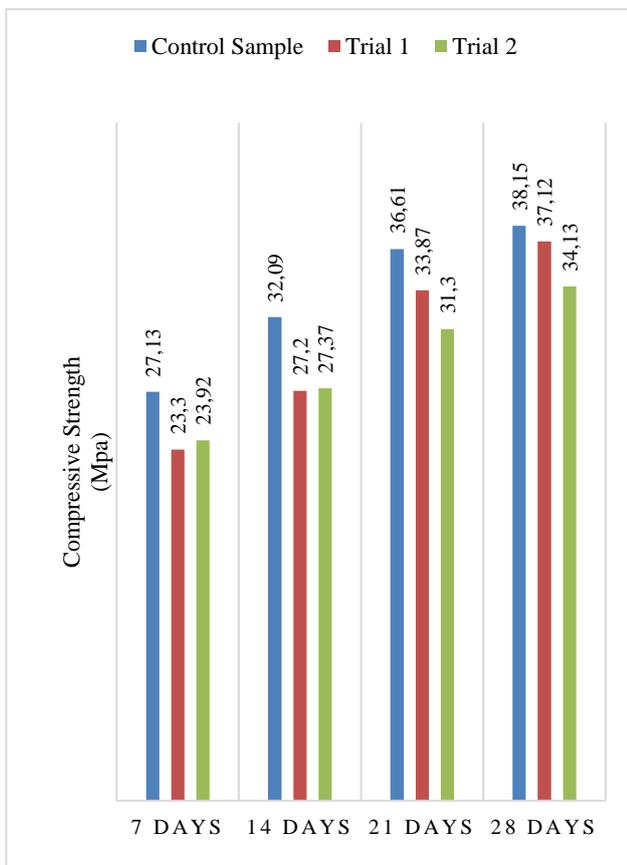
Figure 7: Comparison of Compressive Strength among Control, Trial 1, and Trial 2 Samples
