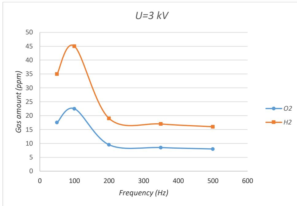
**Figure 3.** Frequency-Gas Quantity characteristic taken at constant voltage  $U=3\text{ kV}$
