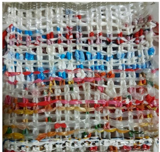
Figure 7. (a, b). Experiment 1, the surface woven by knotting (carpet weaving) technique using grocery bags has a shaggy appearance.
