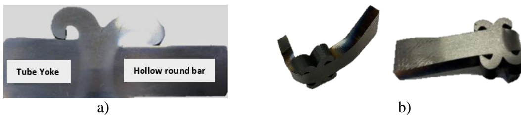
Figure 7. A bended specimen during the bending test to investigate the cross-section of welded joint in terms of the welding quality and performance.
