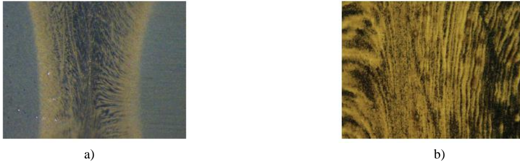
Figure 9. A specimen under microscopic inspections, a) 10x magnification on weld line, b) 50x magnification on weld line
