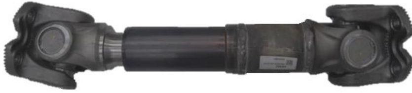
Figure 10. A drive shaft specimen produced for laboratory tests
