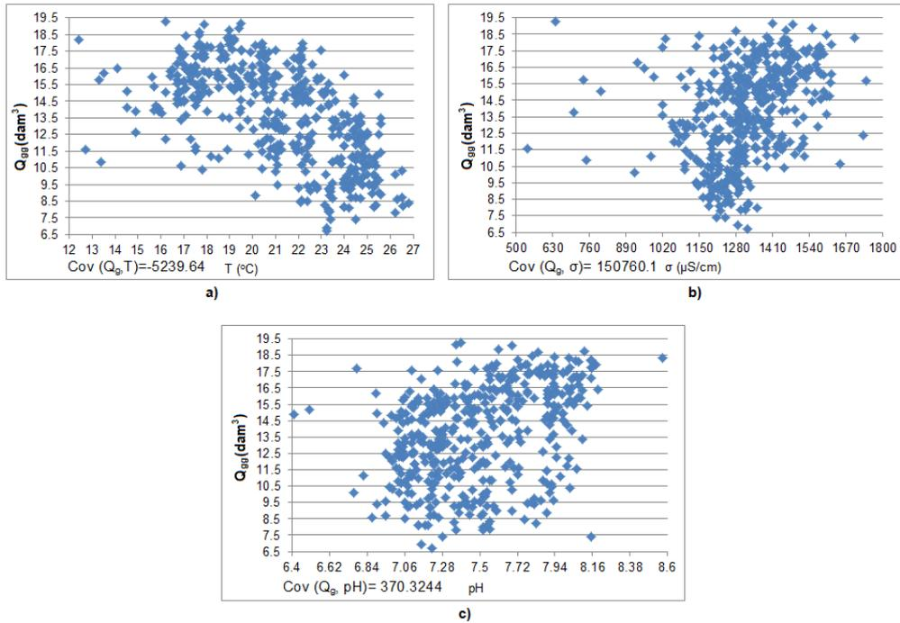
**Figure 9.** The covariance analysis of the physical and chemical properties of the wastewater, **a)** the covariance of daily gas generation ( $Q_{gg}$ ) of the treatment plant shown according to the temperature ( $T$ ), **b)** the covariance of daily gas generation ( $Q_{gg}$ ) of the treatment plant shown according to the conductivity ( $\sigma$ ), **c)** the covariance of daily gas generation ( $Q_{gg}$ ) of the treatment plant shown according to the pH
