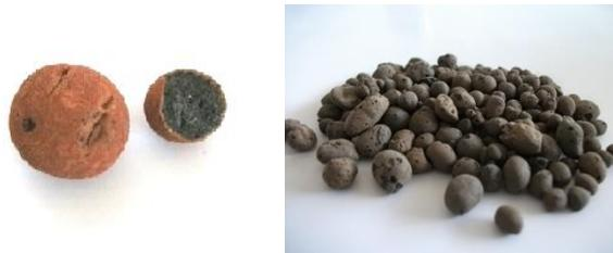
Fig. 1. Expanded clay
