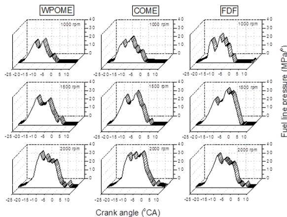
Fig.5. Comparison of the fuel line pressures for test fuels
