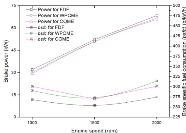
Fig.2. Comparison of the brake power and *bsfc* values for test fuels
