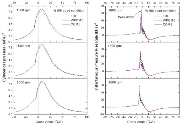
Fig.3. Comparison of the cylinder gas pressures and instantaneous pressure rise rate for test fuels
