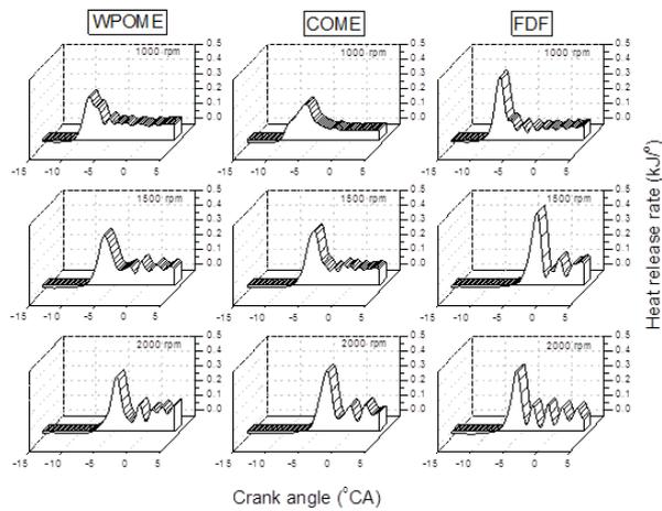
Fig.4. Comparison of the heat release rates for test fuels
