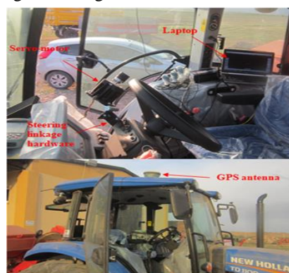
Figure 3 General view of GPS and automatic control system
