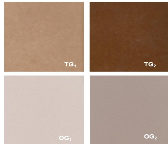
Figure 2. Surface appearance and color of the glazes prepared by neutralized chromite waste, fired at 1200^\circ\text{C} ; \text{TG}_1 , \text{TG}_2 , \text{OG}_1 , \text{OG}_2
