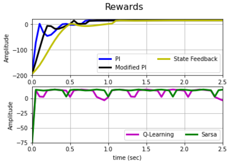
Figure 8. Reward values of Single Tank Liquid Level System by PI, modified PI, state feedback with integral action, Q Learning and SARSA.
