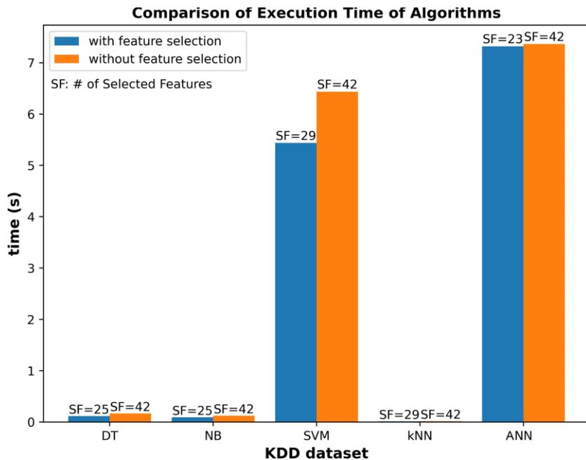
**Figure 7.** Comparison of algorithms in the aspect of execution time on KDD Dataset. Here, the value of the ratio which produces the highest Accuracy value was selected for each algorithm.
