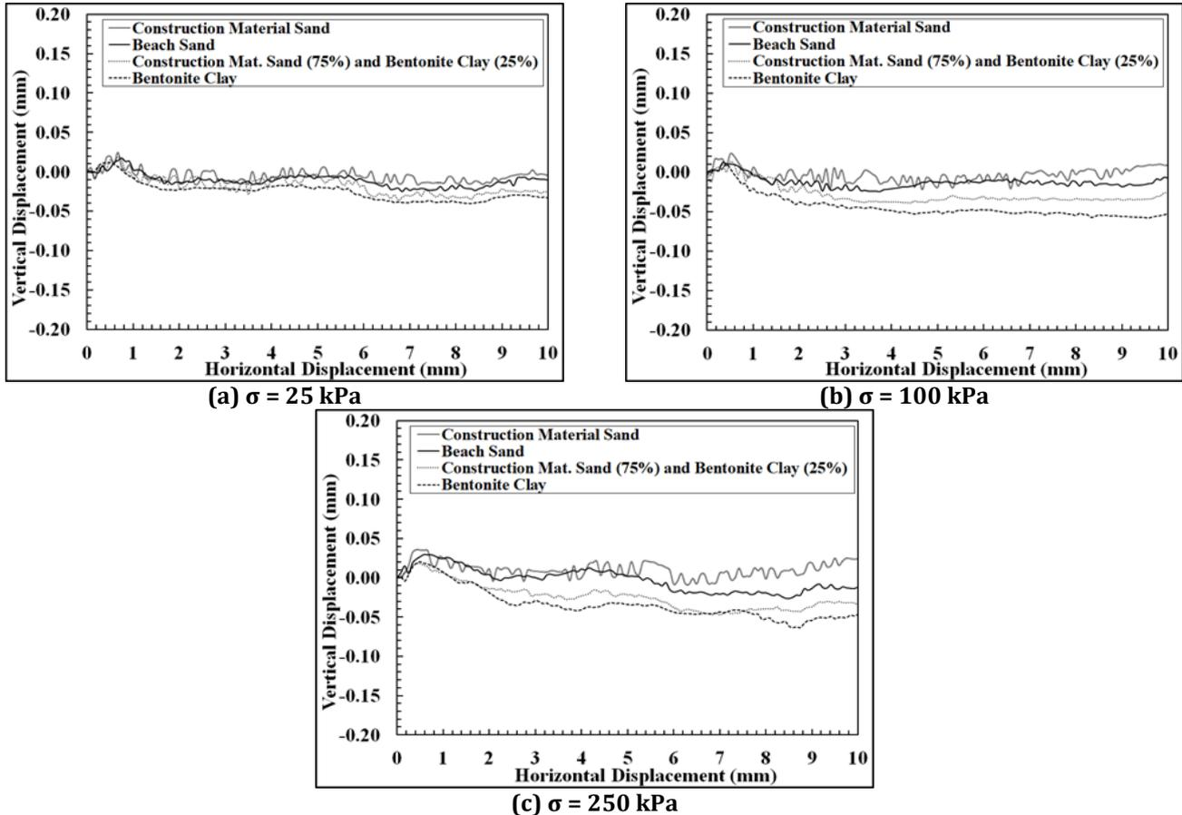
**Figure 5.** The variation in vertical displacement during horizontal displacement mobilized in interface shear tests at different normal loading conditions: **(a)** 25 kPa; **(b)** 100 kPa; **(c)** 250 kPa.
