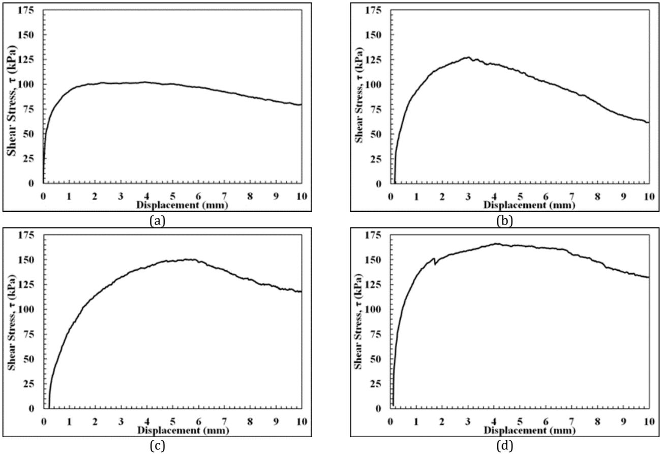
**Figure 4.** Shear response of different interface systems at 250 kPa normal stress level: **(a)** Bentonite clay; **(b)** Bentonite Clay/Construction material sand admixture; **(c)** Beach sand; **(d)** Construction material sand.
