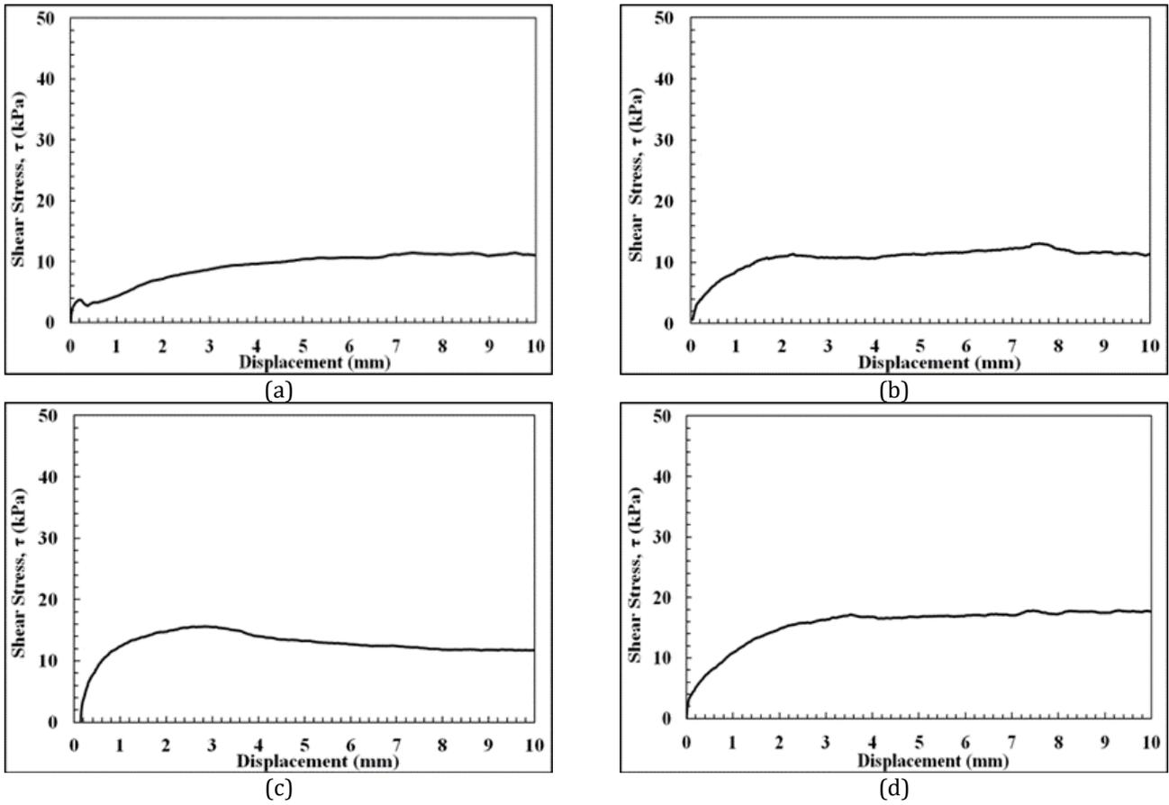
**Figure 2.** Shear response of different interface systems at 25 kPa normal stress level: **(a)** Bentonite clay; **(b)** Bentonite clay/construction material sand admixture; **(c)** Beach sand; **(d)** Construction material sand.
