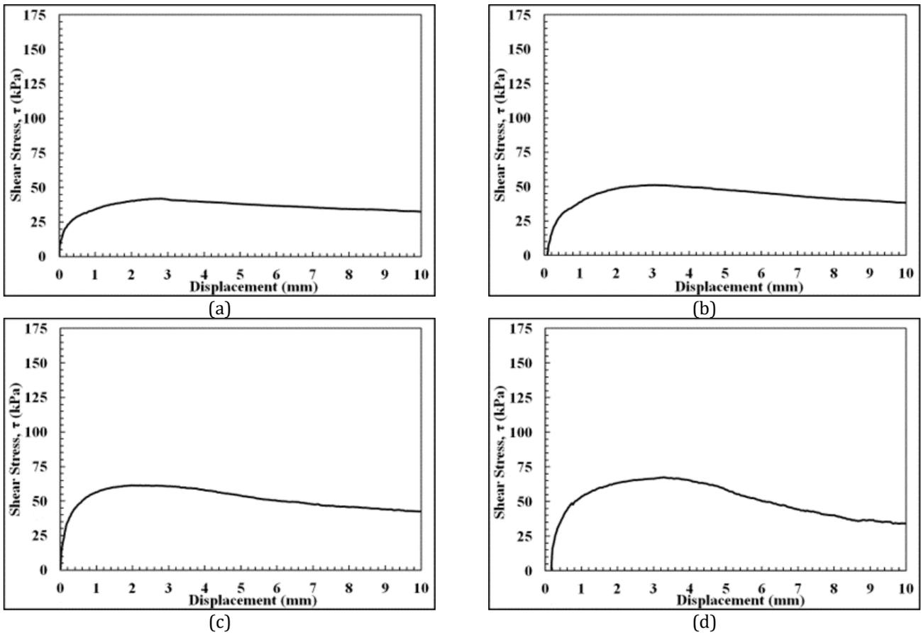
**Figure 3.** Shear response of different interface systems at 100 kPa normal stress level: **(a)** Bentonite clay; **(b)** Bentonite clay/construction material sand admixture; **(c)** Beach sand; **(d)** Construction material sand.
