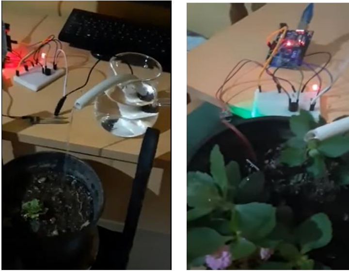
Photo 2. Irrigation system with Arduino
