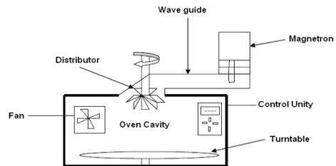
Figure 1. Schematic diagram of the microwave oven
