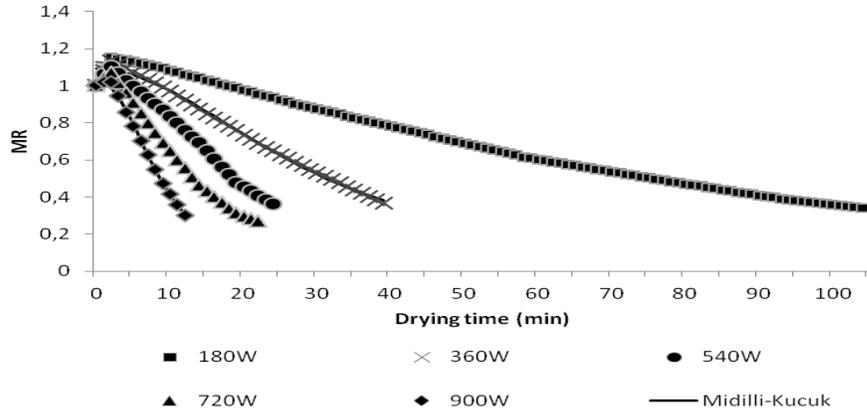
Figure 2. Variation of experimental and predicted moisture ratio by Midilli-Kucuk model with drying time at selected microwave output powers
