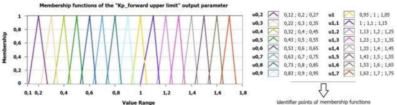
Figure 9. Membership functions and identifier points for the *K<sub>p</sub> forward upper limit* output parameter
