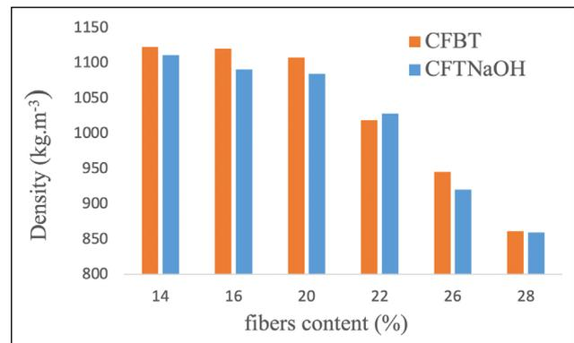
**Figure 6.** Density of concrete as a function of fiber content.
