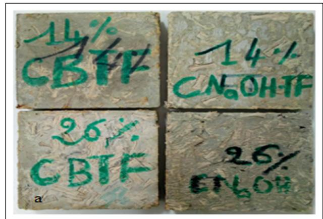
**Figure 1.** Baobab trunk fibers concretes.
