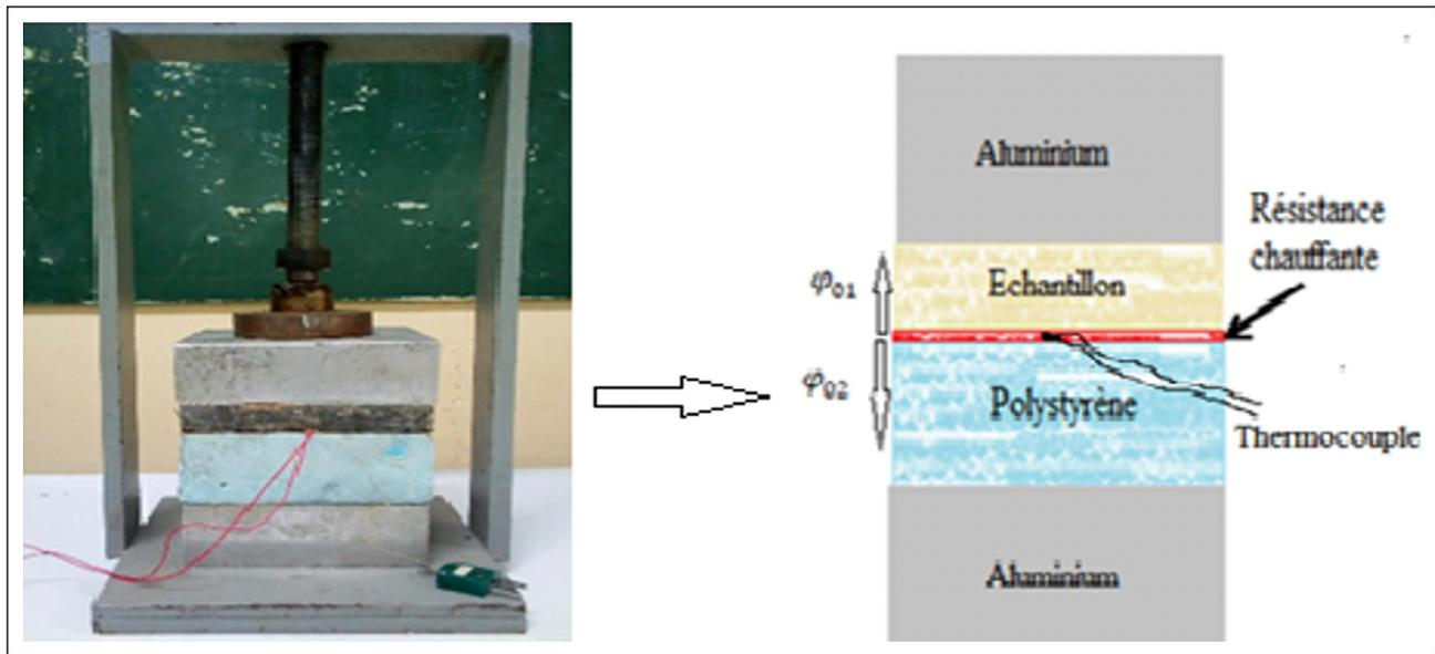
Figure 2. Asymmetrical hot-plane device.
