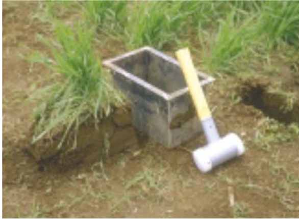
Fig.9. Root box with extracted root-soil monolith together with wheat shoots (Reynolds et al., 2001).
