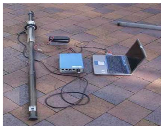
Fig.4. Equipment for root study using the minirhizotron method (Chen, 2011).
