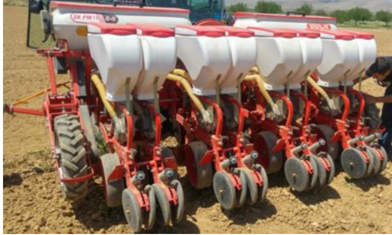
Figure 1. Twin row pneumatic precision seed drill used in the trial
