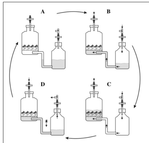
**Figure 1.** Technological design and operating principle of the Twin-Flask bioreactor system: (A) exposure time (B) Displacement of the liquid medium. Air pressure is applied to the media storage tank and the liquid media moves into the culture chamber; (C) immersion time; (D) evacuation of the nutrient medium. The air pressure is turned off and the medium flows back into the middle storage tank due to gravity.
