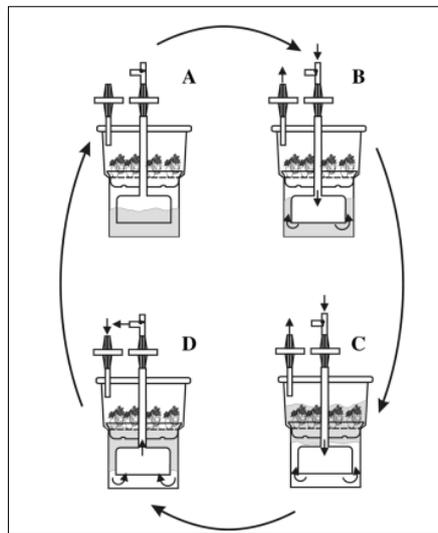
**Figure 4.** Technological design and operating principle of the RITA system: (A) exposure time; (B) Displacement of the liquid medium. Air pressure is applied to the lower chamber through the middle pipe. Liquid media moves to the upper chamber; (C) immersion time; (D) evacuation of the nutrient medium. The airflow is stopped and the medium flows back into the lower chamber due to gravity.
