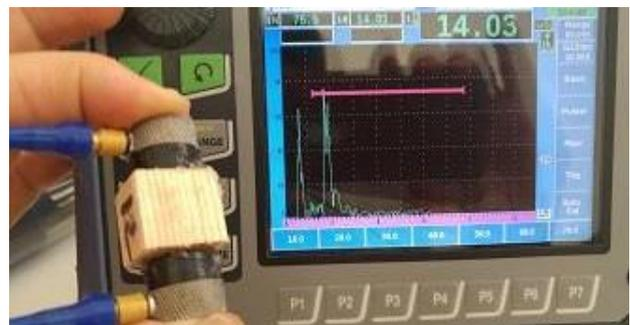
Figure 2. Measurement of sound velocity.
