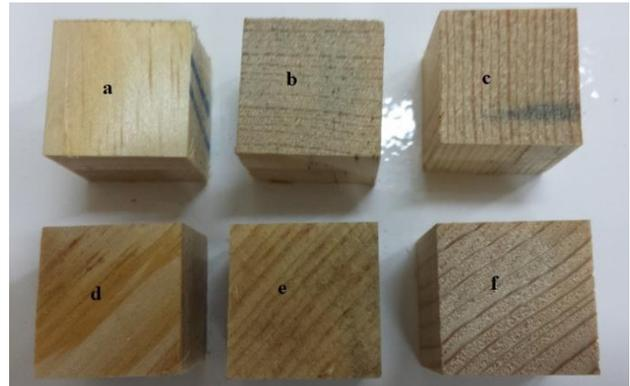
Figure 1. Examples used in measuring ultrasonic sound velocities and determining elasticity constants (a-  $C_{11}, C_{44}$ , b-  $C_{22}, C_{55}$ , c-  $C_{33}, C_{66}$ , d-  $C_{12}$ , e- $C_{13}$ , f- $C_{23}$ )
