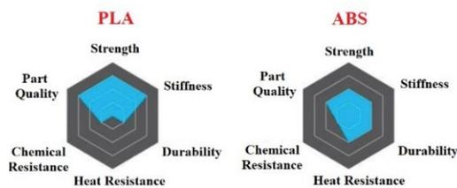
**Figure 1.** Comparison of PLA vs ABS [26].
