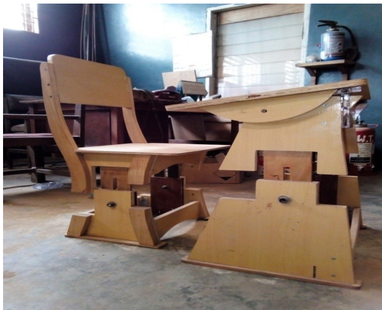
Figure 2. Sitting-posture Measurement Device (Developed by MWP Lab 2015)
