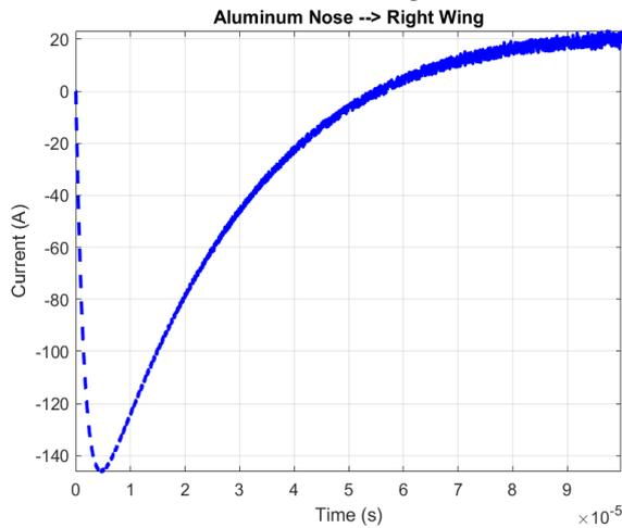
**Figure 8.** Induced current value on unshielded cable
