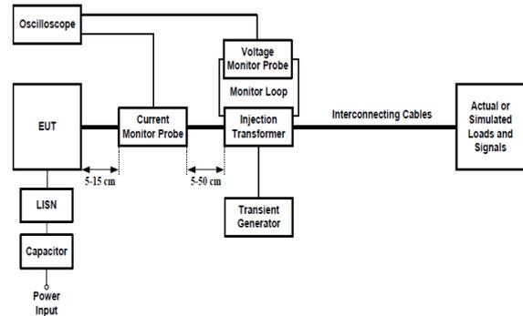
Figure 16. MIL-STD-461G, FIGURE CS117-10, Typical setup for bulk cable injection of lightning transients on complete interconnecting cable bundles
