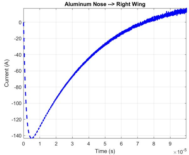
**Figure 10.** Induced current value on the shield
