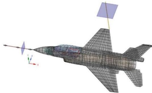
**Figure 5.** In the EMA3D program, the F16 model and lightning attach/de-attach points
