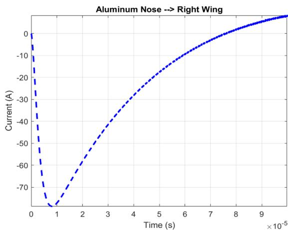
**Figure 9.** Induced current value on shielded cable
