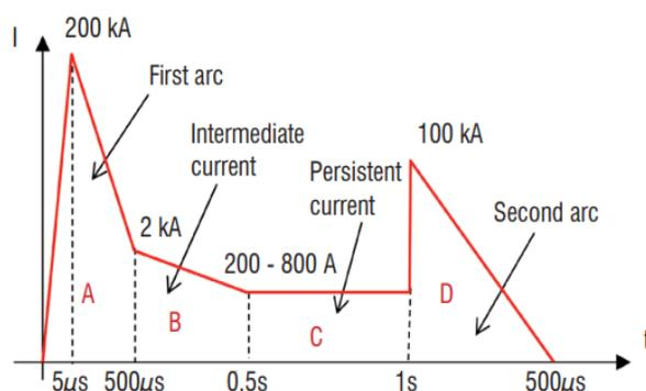
**Figure 1.** Lightning Waveform, as defined in RTCA DO-160 [9]
