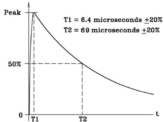
**Figure 22-1** Current Waveform 1
