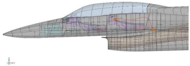
**Figure 6.** Close-up view of the modeled cable in the EMA3D program
