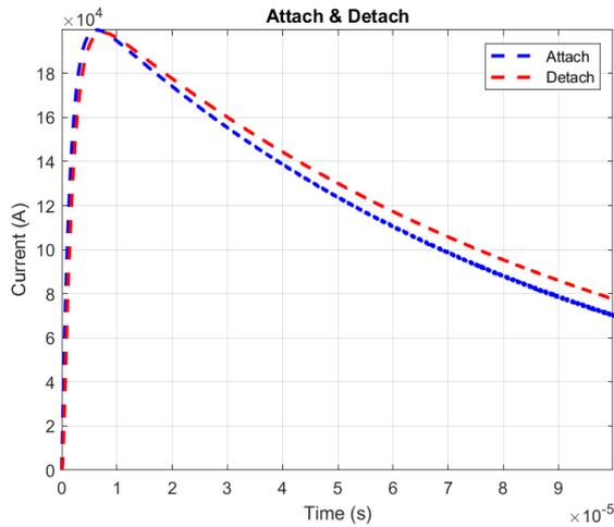
**Figure 7.** Levels of simulated lightning current (Component A) at attach and de-attach points
