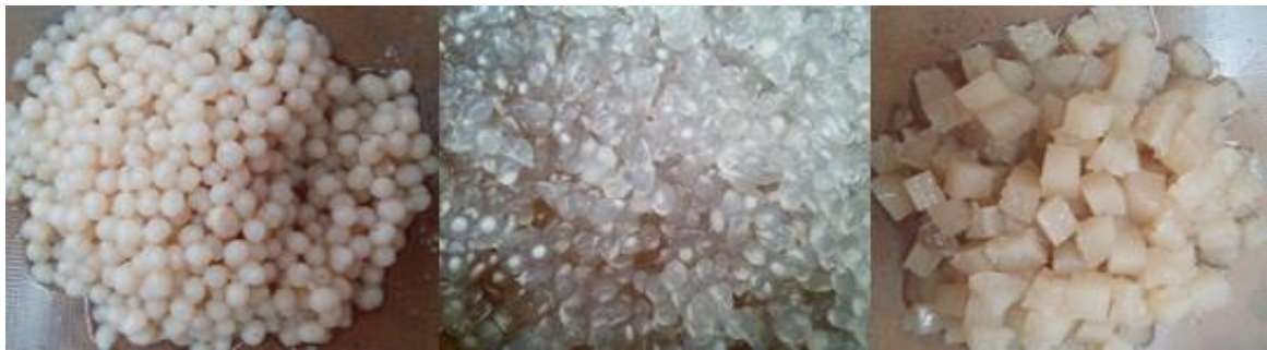
Figure 1: Entrapment immobilization(L), capsulation immobilization (C), gel immobilization (R)
