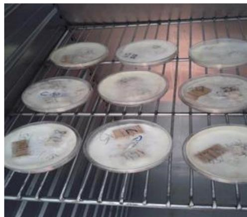
Figure 1. Fungal decay test
