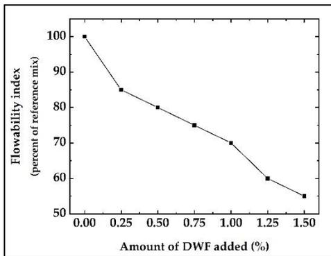
Figure 4. The flow indices of the CLCM batches.
