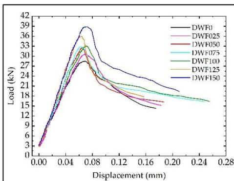
**Figure 11.** Load-displacement plot for DWF reinforced CLCMs.
