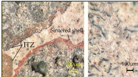
**Figure 6.** Interfacial transition zone of aggregate-cement matrix and DWF-cement matrix
