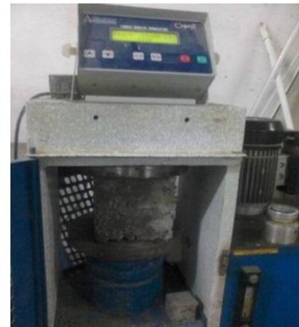
Figure 5: Compressive strength test of the first sample.
