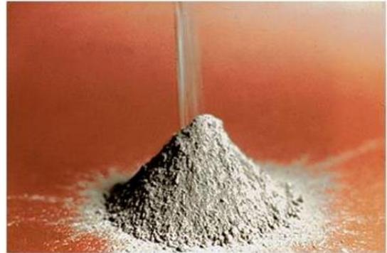
Figure 1: Micro silica used in concrete mix design.
