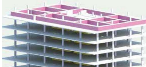
Figure 8. Model of roof high beam system [23]
