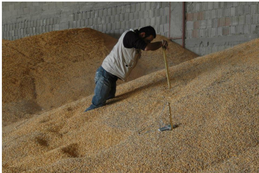
Figure 2. Spiral grain probe used for corn sampling.
