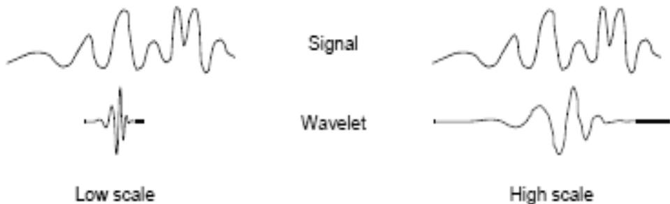
Figure 20- Signal and wavelet in low and high scales
