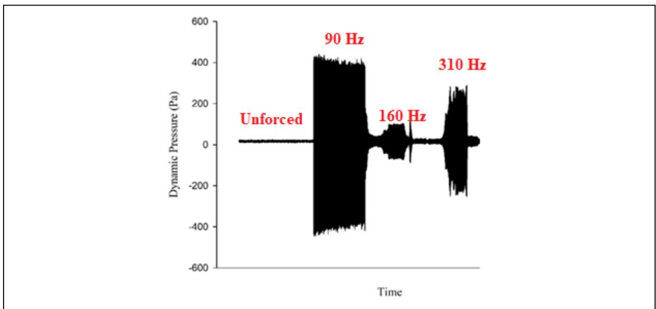
**Figure 7.** Natural acoustic mode of combustion chamber (67% CH<sub>4</sub>-33% C<sub>3</sub>H<sub>8</sub>)
