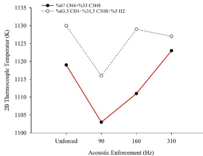
**Figure 4.** 2B thermocouple temperature for different acoustic enforcement
