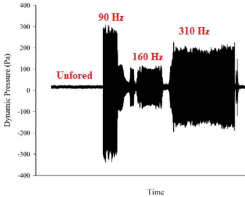
**Figure 6.** Natural acoustic mode of combustion chamber (63,5% CH<sub>4</sub>-31,5% C<sub>3</sub>H<sub>8</sub>-5% H<sub>2</sub>)
