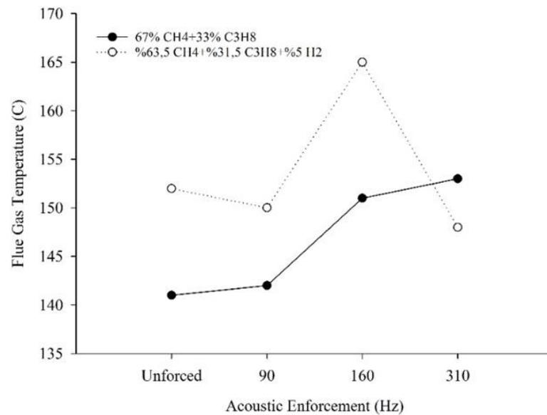
**Figure 5.** 2B flue gas temperature for different acoustic enforcement
