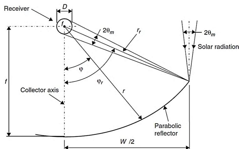
**Figure 2.** Cross-section of a parabolic trough collector [15]
