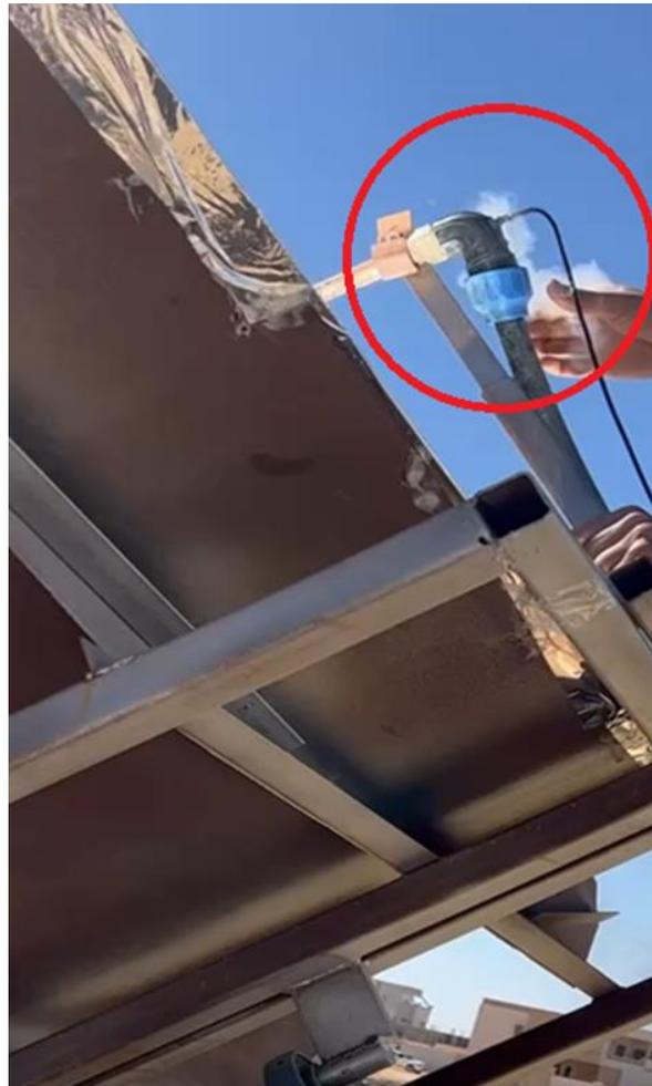
*Figure 6. Steam generated at zero flowrate test*
